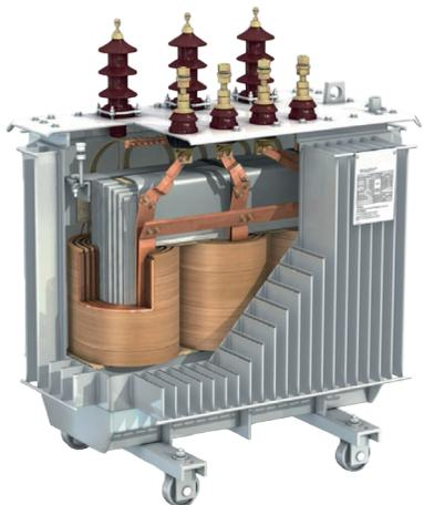
Figure 11 – 18 Common oil-immersed distribution transformer cut view.
